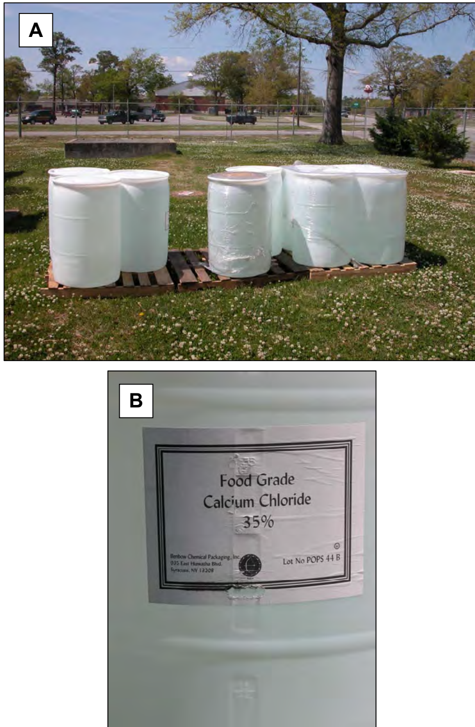
Figure 5. Photographs showing calcium chloride solution to be used for tracer study of the Hadnot Point water-distribution system: (A) 55-gal drums, and (B) label showing 35% by weight.
