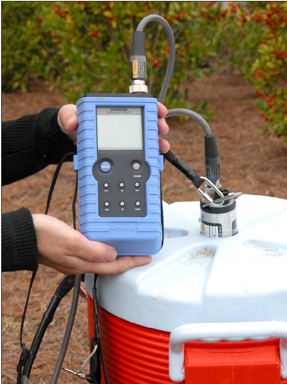
Figure 15. Photograph showing HORIBA W-23XD water-quality control unit and cable attached to dual probe ion detector housed in a protective plastic 5-gallon water jug.
