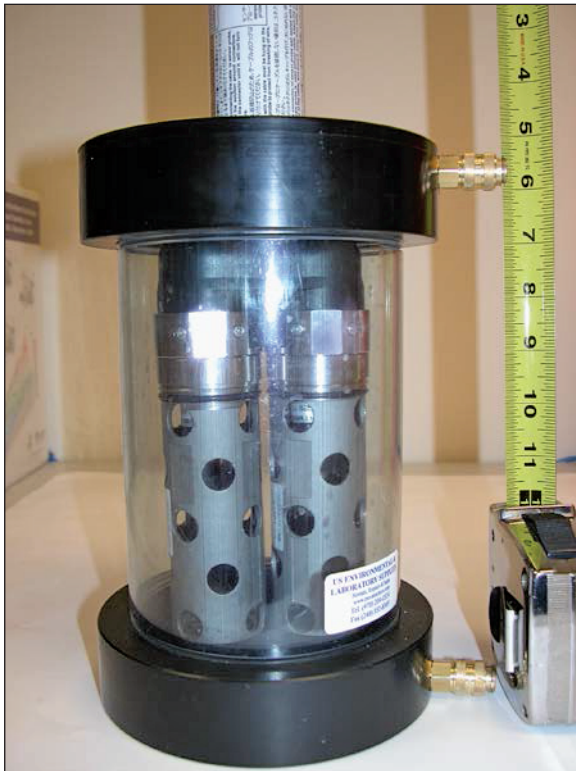
Figure S8.14. Selected field-test equipment: Horiba W-23XD continuous recording, dual-probe ion detector data logger inside flow cell, Hadnot Point–Holcomb Boulevard study area, U.S. Marine Corps Base Camp Lejeune, North Carolina, 2004.
