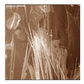
Scanning electron micrograph of asbestiform amphibole
